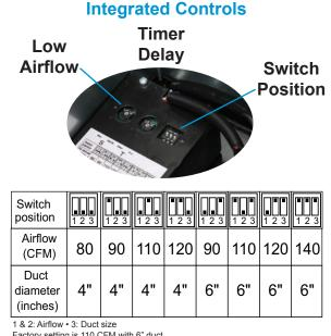
Factory setting is 110 CFM with 6" duct
